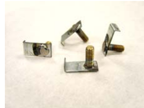
Figure 13 (below): T-bolts for lower hole on brackets.
