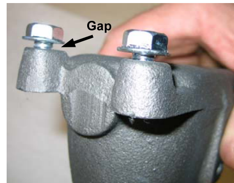
Figure 14: Leave a gap between the screw and the burner surface.
