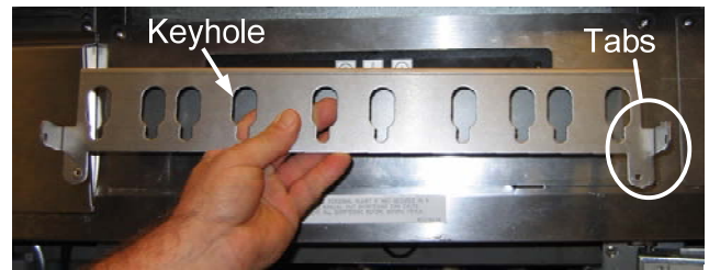
Figure 3: The brace in its final position, as it will look inside of the fryer.
