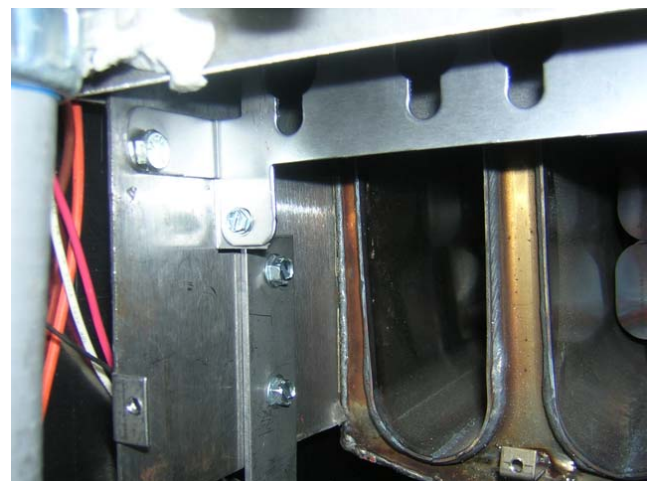
Figure 11: Slide the brace up, flush with the frypot.
